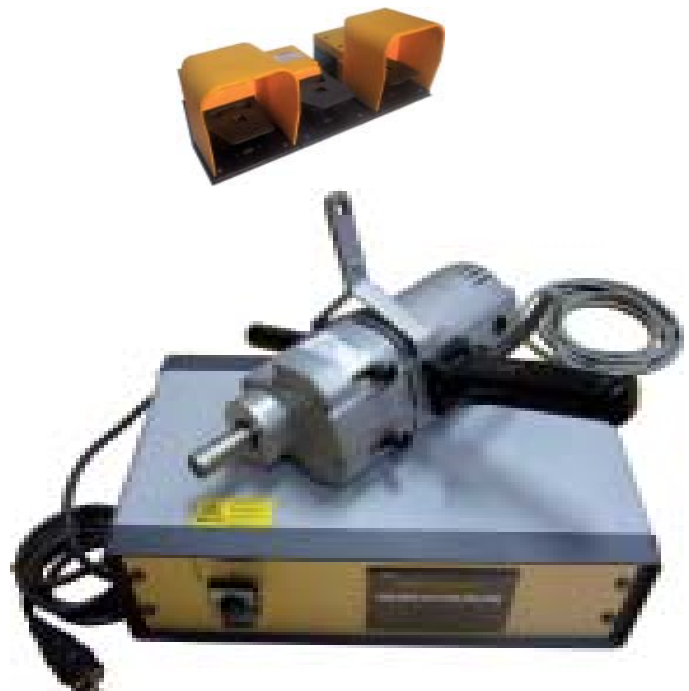
fig.: Expanding controller type NFAB S/2 with driving motor type D 32
