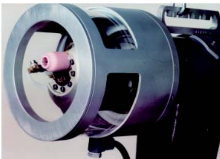
fig.: Orbital-welding head T-250, with double gas shield chamber to weld titanium tubes
