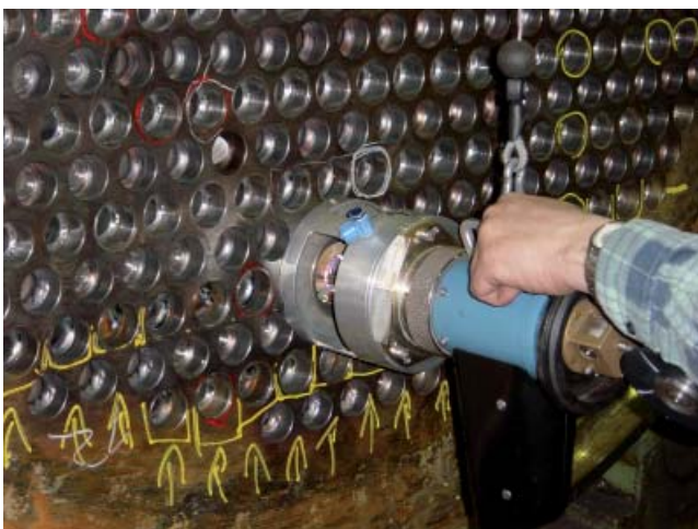
T-250 with standard double gas shield chamber
