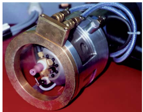
double gas shield chamber, liquid cooled
