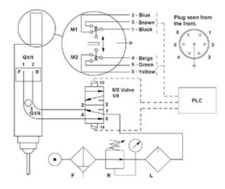
The max load for the switches at 220 V is 1A.
