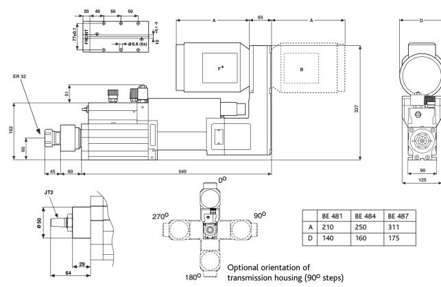
\*Front mount is not possible at BE487 with linear transducer
