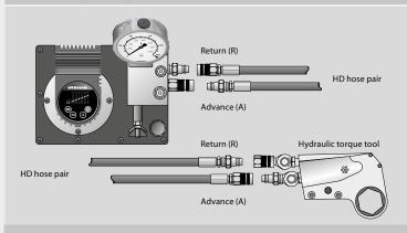
Included in the scope of delivery: hydraulic hoses, 5 m long (DN 6)
