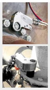
*alkitronic® NOVA* hydraulic pump Depending on model up to 4 hydraulic wrenches can be operated at the same time. *alkitronic® NOVA specials*
