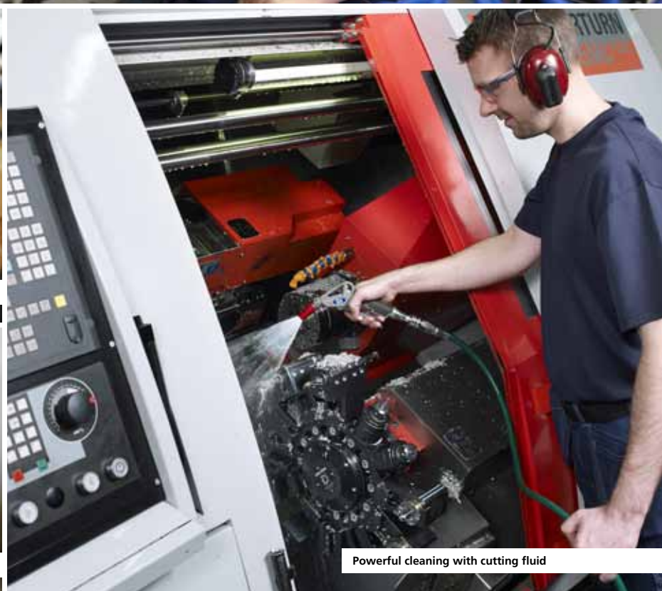
High thrust/blow force for removing chips
