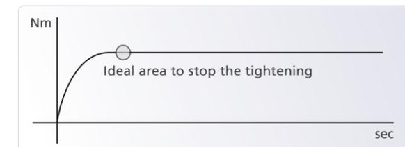
Impulse wrenches archive the highest quality joint if the tightening is finished in this area (horizontal part of the torque curve)
