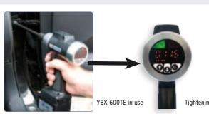
The YBX-600T and YBX-800T are Electronically Controlled battery impulse wrenches with integrated angle encoder for highly accurate torque tolerances. The shut-off is calculated over several impulses. The controller is integrated and enables counting, Poka Yoke.
