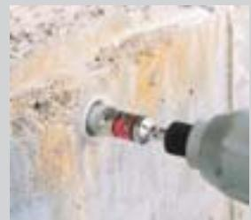
Use for setting and pulling plastic cones in form work.
